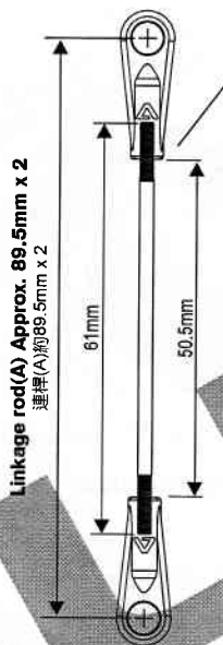
Linkage rod (A) 連桿(A) \phi 2.5 \times 61 \text{mm}
